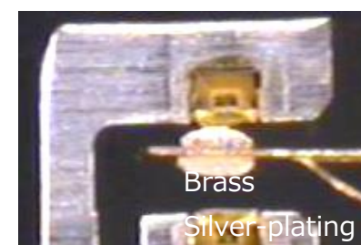
Fixed Contacts with Gold-plating
