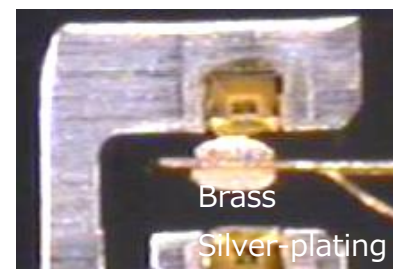
Fixed Contacts with Gold-plating
