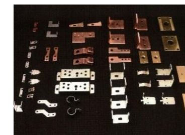
Stamping Parts (Shaving Process) Outer Diameter Stamping, Punching, and Tapping
